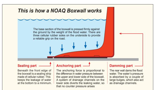
Each box consists of a damming part (the rear wall), an anchoring part (the horizontal section that rests on the ground) and a sealing part (the front edge of the horizontal section). Sealing strips of cellular plastic are fitted under the front and side edges. Each box is also fitted with a pair of cellular rubber soles to create a good grip on the road.
